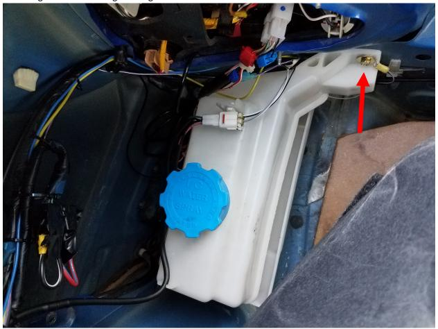
4) Back at the time/relay, Run the switch connector end of the harness down the kick panel under the carpet and behind the radio/ climate control. Then over around the back of the fuse box, so the wires come out to the left of the fuse box. Make sure the wiring does not interfere with the peddles.
