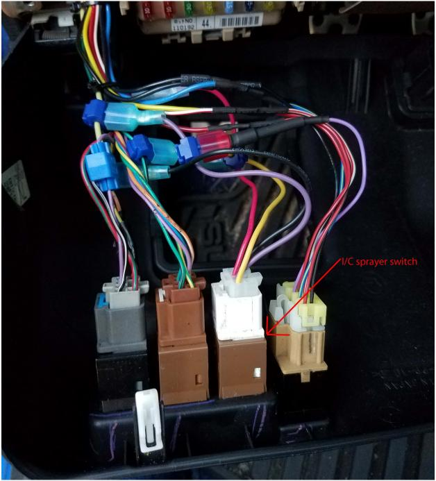
7) Locate the fog light switch connector. (even if you don't have fog lights you should have the fog light switch harness siting in one of the dash blanks) use the included Red T-taps on the
