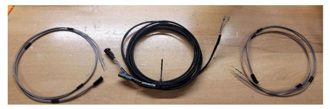
The 2 door harnesses do not have loom on them to aid in pulling the wires thought the rubber door wire tubes. Its best to use some type of wire snake or stiff wire.
